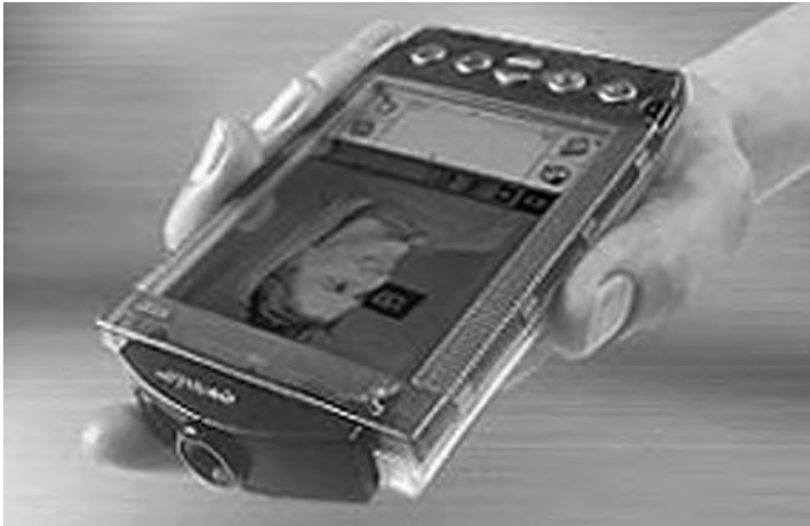
FIGURE 12. The Handspring Visor PDA with the Eyemodule Camera. This handheld device blurs the distinction between computational device, Personal Digital Assistant (PDA) and digital camera (< http://www.handspring.com >).
