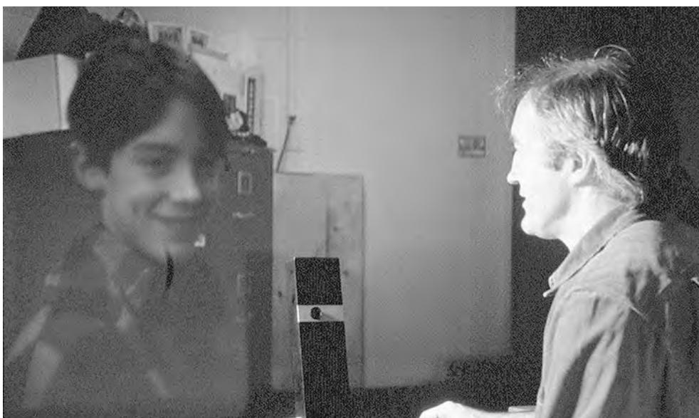
FIGURE 10. Face-to-Face. In this scenario, each participant has a computerized desktop on which the same information is displayed. The intention is to capture the essence of working across the desk from one-another. Each sees the remote participant life-size. The video camera (from a Hydra unit) is unobtrusive on the desk. Participants interact with the computer using a stylus. When one participant looks down to their desktop, their eyes seem to project into the space of the other, thereby strengthening the sense of Telepresence. While there is a considerable amount of technology involved, it is integrated into the architectural ecology. What one gets is lots of service and lots of space, not lots of gear and appliances. Photo: Ontario Telepresence Project.
